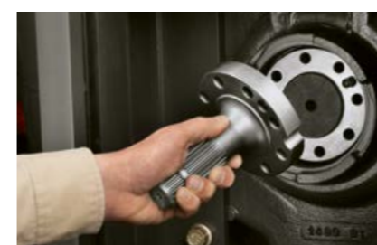
The PTO stub can be changed easily
