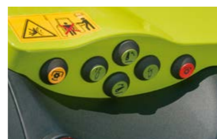
External controls for rear PTO on both mudguards
